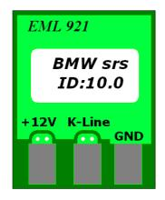
+12V - Power supply K-Line - data line GND - Ground
