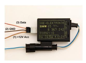
In the picture is shown the original sensor control unit, located at the bottom of the passenger front seat.
