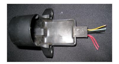
Cut wires from immobilizer mounted on the ignition lock.
