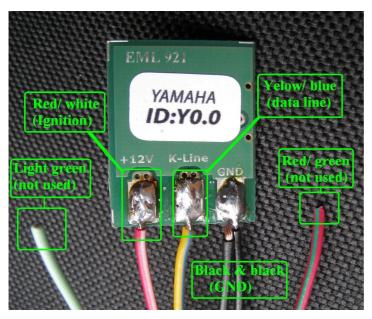
Connect emulator to wires (bike side) according colors shown in picture
