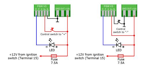
FSW V3 control switch can be connected to plus (+) or to minus (-).
