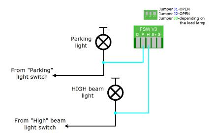
NOTE: When HIGH beam signal no need, "H" input can be not connected, connect only "P" input.
