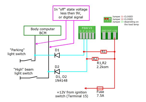
NOTE: When HIGH beam signal no need, "H" input can be not connected, connect only "P" input. If HIGH beam signal not connected, J2 jumper MUST BE OPEN and resistor R2 not connected.
