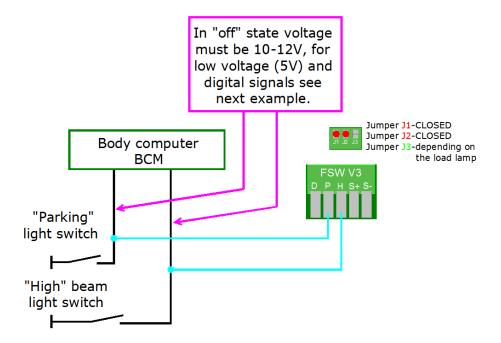
NOTE: When HIGH beam signal no need, "H" input can be not connected, connect only "P" input. If HIGH beam signal not connected, J2 jumper MUST BE OPEN!
